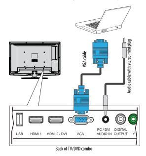
3 Connect an audio cable with a stereo mini plug (not included) to the **PC/DVI AUDIO IN** jack on
